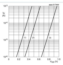
$T_i = 25 \,^{\circ}C; \, V_{DS} = 5 \,^{\circ}V$
