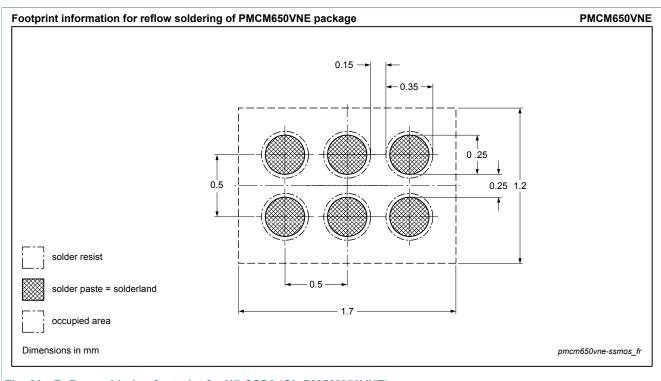
Fig. 20. Reflow soldering footprint for WLCSP6 (OL-PMCM650VNE)
