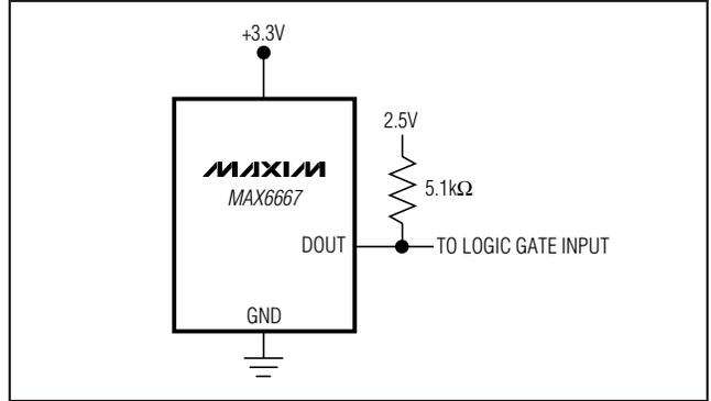
Figure 4. Low-Voltage Logic
