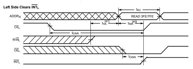
$<sup>\</sup>begin{array}{l} \textbf{Notes} \\ 40. \ \text{Parameter} \ t_{\text{INS}} \ \text{or} \ t_{\text{INR}} \ \text{depends on which enable} \ \text{pin} \ (\overline{\text{CE}_L} \ \text{or} \ R \overline{\text{W}_L}) \ \text{is asserted last.} \\ 41. \ \text{Parameter} \ t_{\text{HA}} \ \text{depends on which enable} \ \text{pin} \ (\overline{\text{CE}_L} \ \text{or} \ R \overline{\text{W}_L}) \ \text{is deasserted} \ \text{first.} \end{array}$
