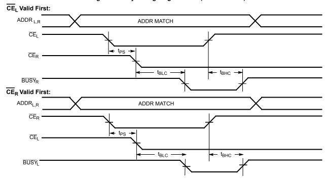
Figure 10. Busy Timing Diagram No. 2 (ADDR Arbitration) [37]
