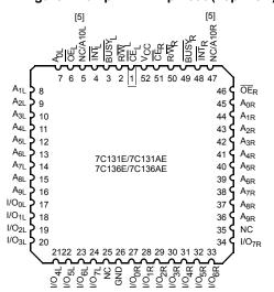
Figure 2. 52-pin PQFP pinout (Top View)
