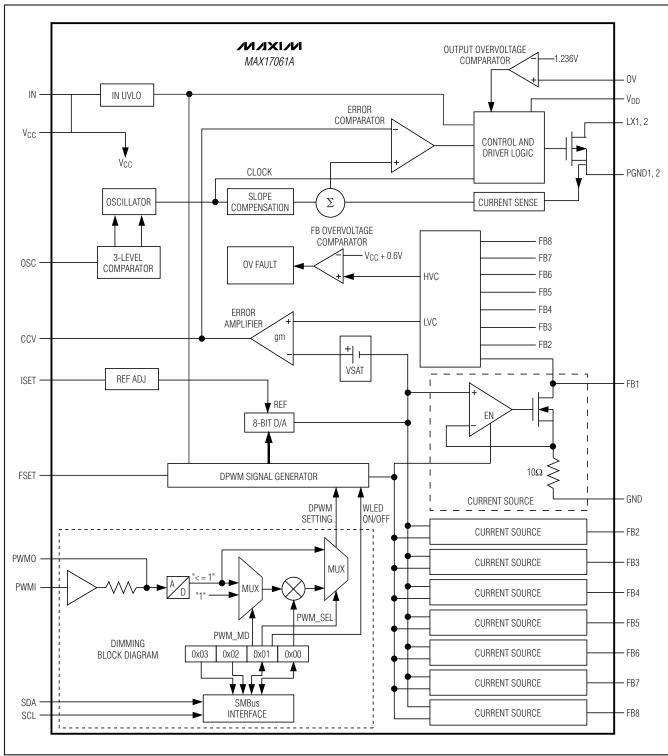
Figure 2. Control Circuit Block Diagram
