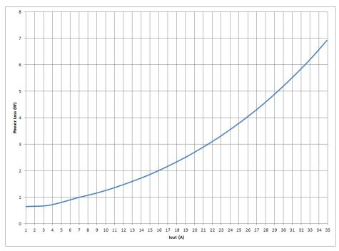
Figure 54: Power loss versus load current
