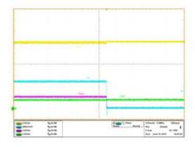
$\begin{array}{c} \text{Figure 44: Operation 00, Immediate OFF, 35A} \\ & \text{load} \\ & \text{Ch}_{\text{1}}\text{:P}_{\text{Vin}}, \text{Ch}_{\text{2}}\text{:V}_{\text{out}}, \text{Ch}_{\text{3}}\text{:P}_{\text{Good}}, \text{Ch}_{\text{4}}\text{:Enable} \end{array}$
