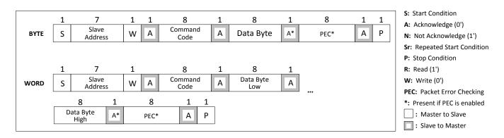
Figure 58: SMBus Write Byte/Word
