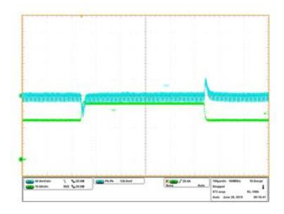
Figure 50: Transient Response, 24.5A to 35A step (2.5A/us)  ${\rm Ch_1:V_{out},\,Ch_4:I_{out}}$
