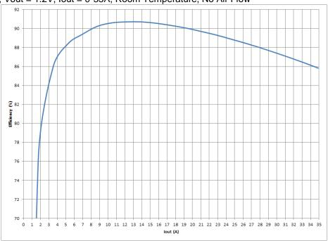
Figure 53: Efficiency versus load current
