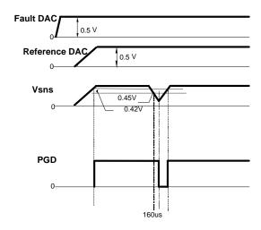
Figure 29: Non-sequenced, Non-tracking Startup
