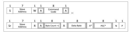
Figure 61: SMBus Block Read with Byte Count=1
