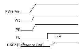
Figure 13: Recommended startup for Normal operation
