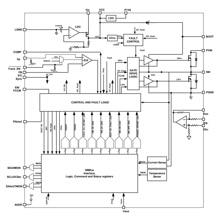
Figure 4: IR38064 Simplified Block Diagram
