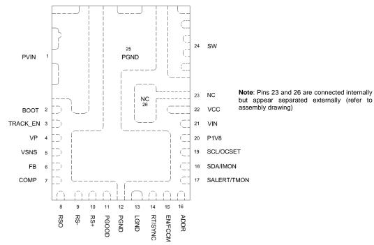
Figure 3: IR38064 package (Top View) 5mm x 7mm PQFN
