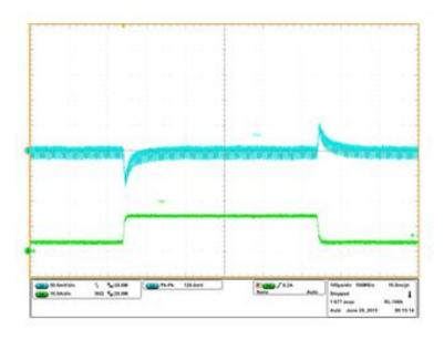
Figure 49: Transient Response, 3.5A to 14A step (2.5A/us)  $Ch_1:V_{out}, Ch_4:I_{out}$
