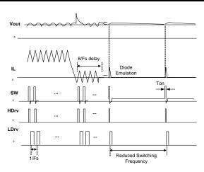
Figure 25: Timing Diagram for Reduced Switching Frequency and Diode Emulation in Light Load Condition (AOT mode)
