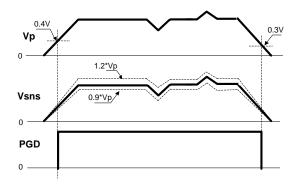
Figure 30: Vp Tracking (Track\_En = 0V)
