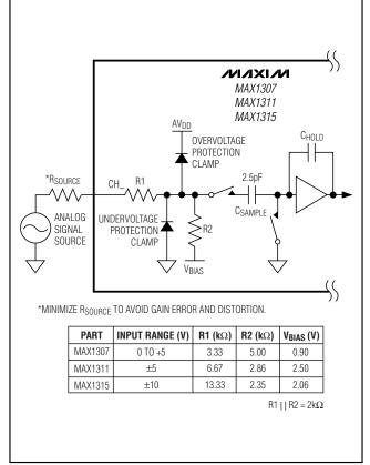
Figure 5. Equivalent Analog Input T/H Circuit
