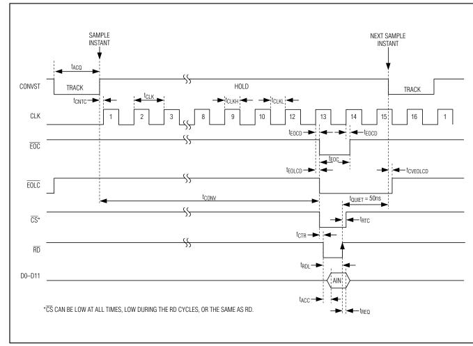
Figure 7. Reading a Conversion—External Clock
