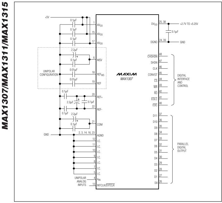
Figure 4. Typical Unipolar Operating Circuit
