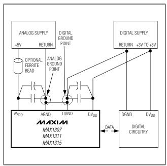
Figure 11. Power-Supply Grounding and Bypassing
