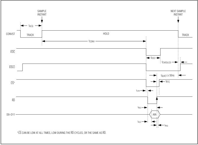
Figure 6. Reading a Conversion—Internal Clock
