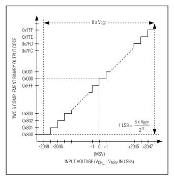
Figure 10. ±10V Bipolar Transfer Function
