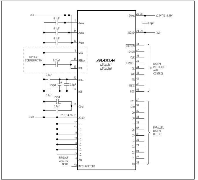
Figure 3. Typical Bipolar Operating Circuit
