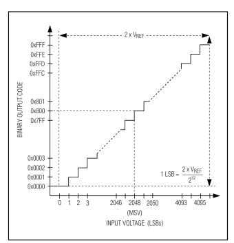
Figure 8. 0 to +5V Unipolar Transfer Function
