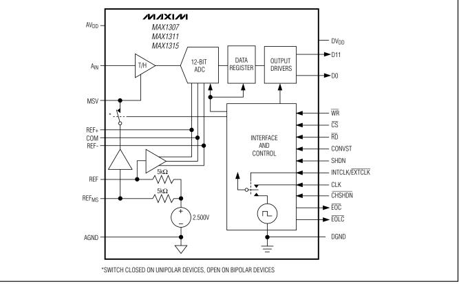
Figure 2. Functional Diagram
