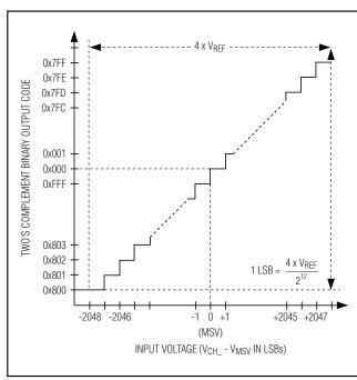
Figure 9. ±5V Bipolar Transfer Function
