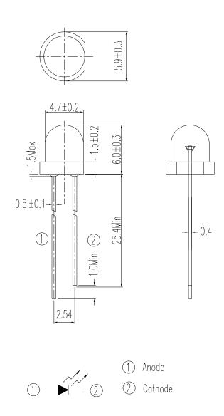
Note: Tolerances unless dimensions ±0.25mm
