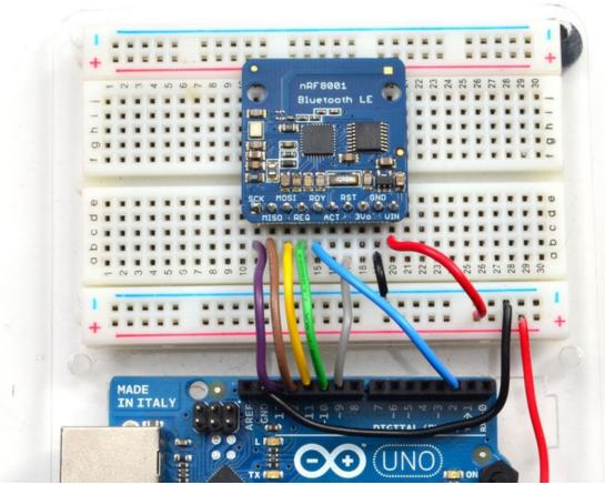
The nRF8001 differs from a classic SPI bus since CS is replaced by two pins, REQ and RDY, but you can still use HW SPI since CS is normally controlled purely in SW anyway.
