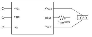
Figure 2. Trim connections to decrease output voltage using fixed resistors
