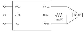
Figure 1. Trim connections to increase output voltage using fixed resistors
