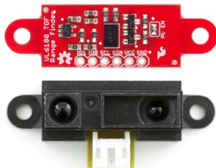
VL6180 Sensor and Sharp GP2Y0A41SK0F Comparison
