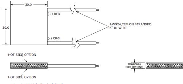
Ceramic Material: Alumina(Al2O3) Solder Construction: 232°C SbSn
