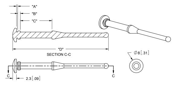
FM-5: TO PULL THROUGH A 3.5±1[.138±.039] HOLE, WITH MAXIMUM 0.8 [.031] PANEL AND 20±0.5 [.787] FAN THICKNESS.
