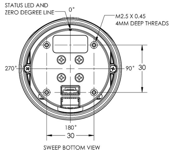
Figure 7, Sweep Mounting Features (all dimensions in mm)
