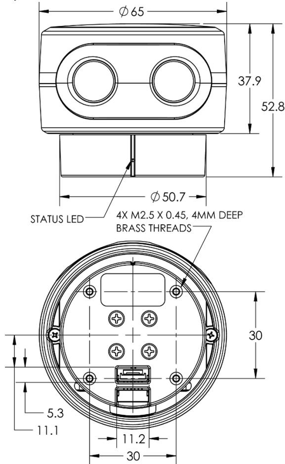
ALL DIMENSIONS ARE IN MM, DRAWINGS ARE NOT TO SCALE
