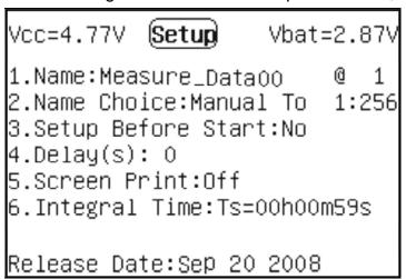
At the top of the screen, it displays the battery voltage and back-up battery voltage separately. The value is calculated in Volts with two decimal digits. In case that the voltage is over 10 V, the screen will display "Over".
