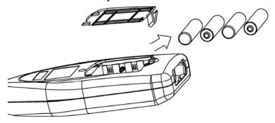
Fig. 3: Opening and closing of battery cover
