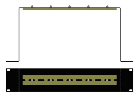
Most N-Tron<sup>TM</sup> products are designed to be mounted on industry standard 35mm DIN rail. However, DIN rail mounting may not be suitable for all applications. Our Universal Rack Mount Kit (P/N: URMK) may be used to mount the 100 Series enclosures to standard 19" racks as an option.
