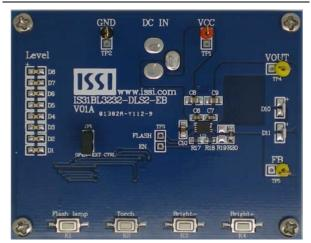
Figure 1: Photo of IS31BL3232 Evaluation Board
