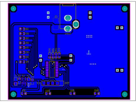
Figure 6: Board PCB Layout-Bottom Layer
