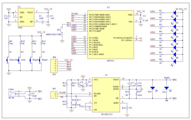
Figure 2: IS31BL3232 Application Schematic
