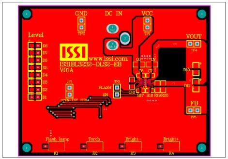
Figure 4: Board PCB Layout- Top Layer
