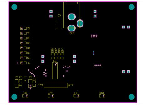
Figure 5: Board Component Placement Guide -Bottom Layer
