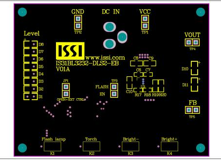
Figure 3: Board Component Placement Guide -Top Layer
