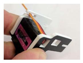
U-Turn the wires at the rectangular holes on plate (do not insert through those holes).
