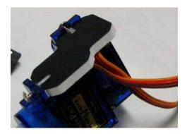
Note that while mounting servos, the Front mount plate (plate C) is on the side of servo wires, as in adjacent picture.
