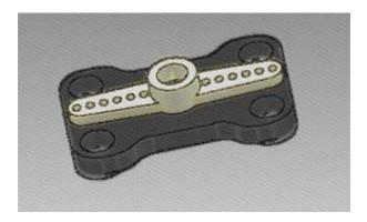
Affix servo horn as shown (with screws from bottom)
