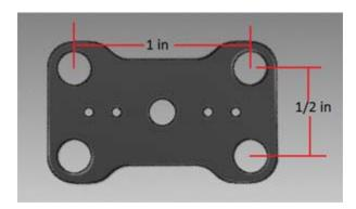
Spacing on this plate is as seen in adjacent picture: (hole size 3/16") Use this spacing to make holes on your target mount plate.
