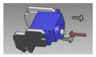
Attach the mount plates C and D to one of the servos and fasten the servo screws  $(\mathbf{W})$ , (do not overtighten).
