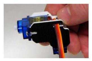
Tuck the servo wires through the holding slit on the mount plate D. The Servo head assembly is ready now.
