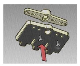
Affix the horn to Plate B as shown below, use screws ( $\mathbf{Z}$ ). Ensure to affix horn on White side of Plate B.
