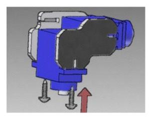
Attach the second servo, and fasten servo screws (W).
