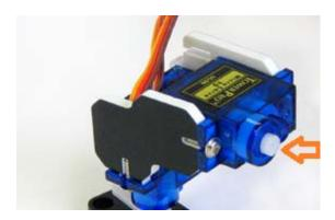
Note the servo on which the camera head will be mounted (Orange arrow).
