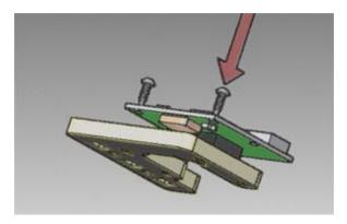
Fasten 2 (Y) screws to plate A in the corner holes, as shown.
