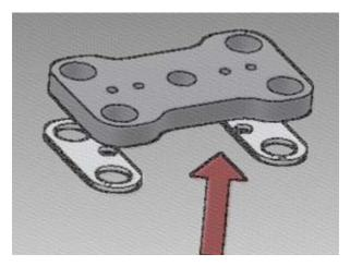
Affix the spacers on the mount plate as shown in adjacent picture and press firmly.
