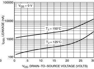
Figure 6. Drain-to-Source Leakage Current vs. Voltage
