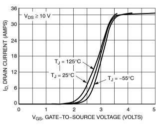
Figure 2. Transfer Characteristics
