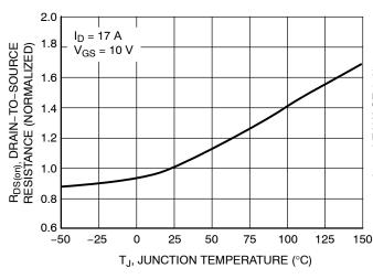
Figure 5. On–Resistance Variation with Temperature
