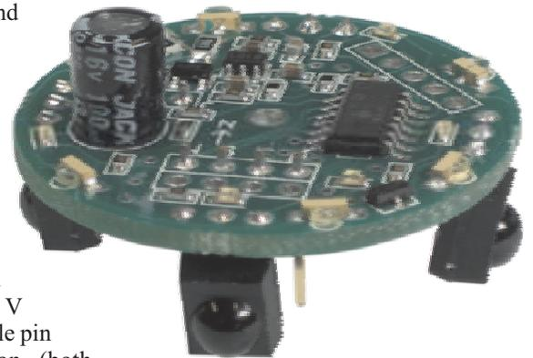
There are two sets of electrical connections to the IR beacon. Three pins on the "west" side are for power and an optional enable input. Apply 6-16 V across the + and - pins; making the enable pin high (5 V) will enable the beacon (both transmission and reception). The four directional outputs are located on the "south" side of the PCB. Each pin is normally high (5 V), and it will go low (0 V) if the other beacon is detected in the corresponding direction.
