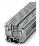
1-level terminal block with double connection on both sides, with built-in resistor 5.1 k $\Omega$ ,  $\pm 0.1\%$ , 0.6 W, cross section: 0.2 ... 2.5 mm², width: 6.2 mm, color: gray
