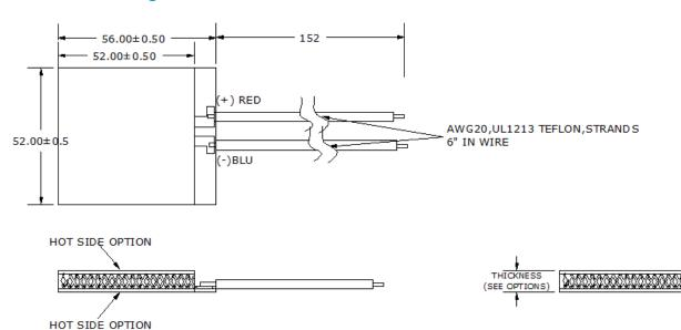
Ceramic Material: Alumina(Al2O3) Solder Construction: 232°C SbSn
