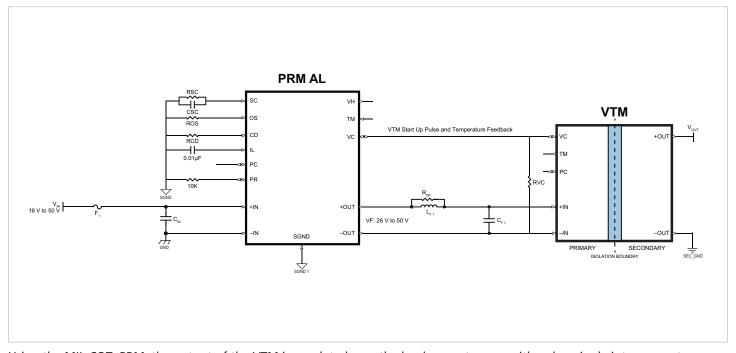
Using the MIL-COTs PRM, the output of the VTM is regulated over the load current range with only a single interconnect between the PRM and VTM and without the need for isolation in the feedback path.
