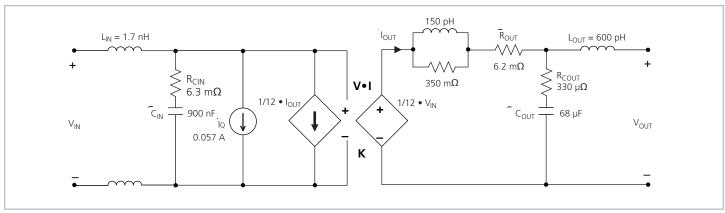
Figure 1 — VI Chip® module AC model (MVTM48EH040M025A00 shown)
